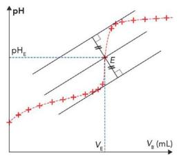
The pH-metric titration curves (pH =  $f(V_{Badded})$  gives the variations in pH as a function of the volume of titrant solution poured show sudden jumps in pH at the equivalence.
